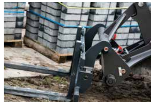
Attachments are fitted safely and easily using the quick coupler.
