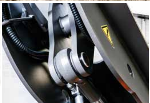
Internal single arm hosing and wiring protects key components.
