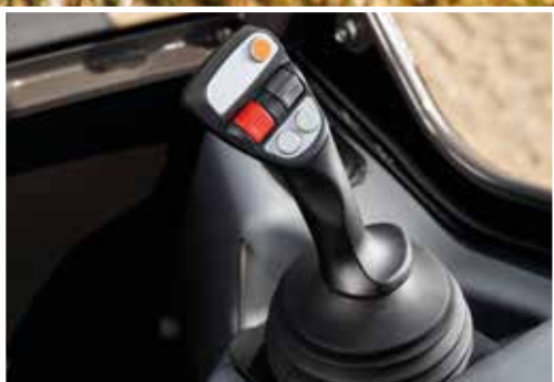
User-friendly controls enhance operator comfort (multifunctional lever is optional).
