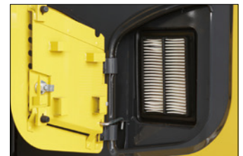
External air conditioner filter
