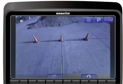
Rear view image on monitor.
