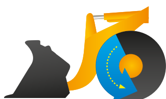
No pressure on the inching/brake pedal: maximum power for traction.
