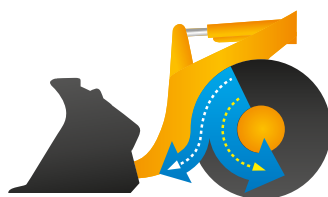
Normal pressure on the inching/brake pedal: the speed reduction, the more power the hydraulic system service.
