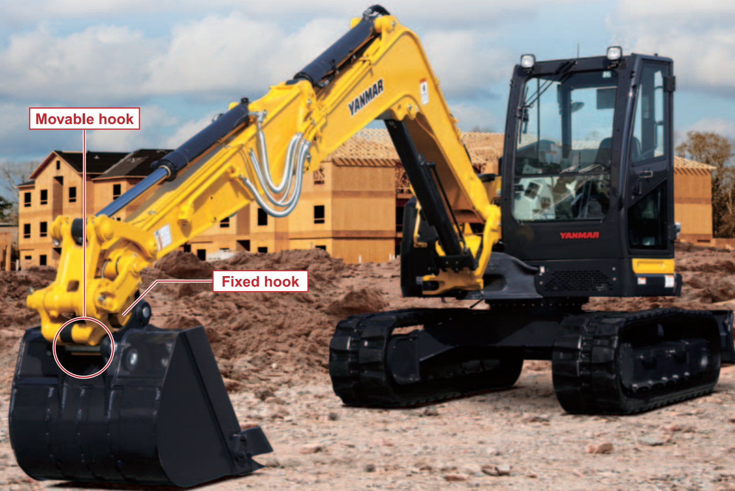
Apply the fixed hook Make the bucket level. Turn the switch to mounting Insert the safety lock pin and fasten.
