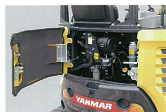
With one touch operator can access to major components for maintenance
