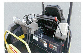
Maintenance of engine became easier than ever, just lift the seat.
