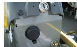
External Power Supply
