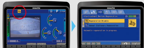
Aftertreatment device regeneration screen
